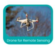
Moreover, the UAV can survey over larger distances than individuals and limit their exposure to hazardous smoke. Finally, drones can also be used to remotely set prescribed burns without human labor or health risk, such as through incendiary payload
